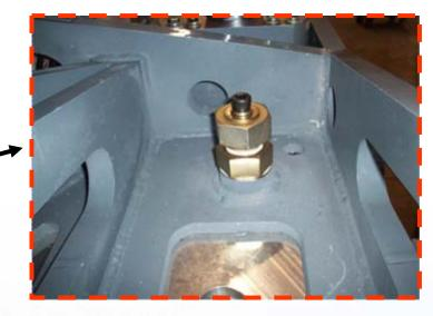
Product adjustment bolts allow for "NO shim" platen adjustment and fine tuning of product sizes.
